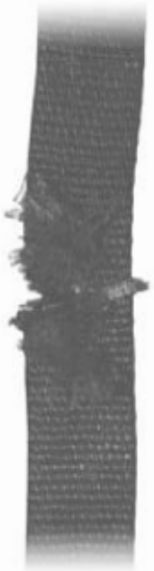
Damage from Unprotected Edges
